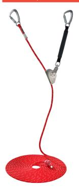
Synchronized retaining clamp with integrated shock absorber attached inseparably to the work rope and serves as a fall stop. It displaces up and down freely except that it will block during a possible fall. Standard supply consists of: Model GRIP 12 complete with integrated shock absorber, supporting rope of 40 cm, carbine with hook and a work rope having a carbiner hook at one end and a knot at the other one.
